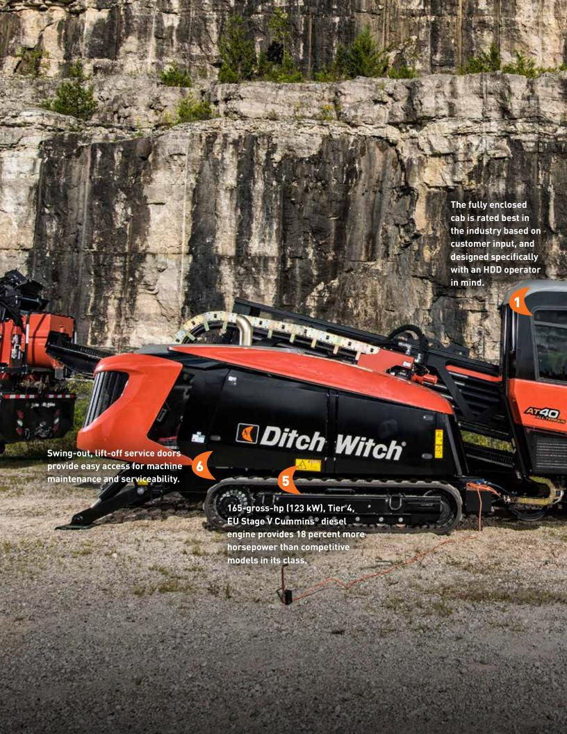
Optimized for industry-leading performance and productivity in hard rock conditions, the Ditch Witch® AT40 All Terrain directional drill is designed with an advanced version of the proven Ditch Witch All Terrain drilling system. The updated, two-pipe system offers boosted power to the bit. Patented design enhancements increase cycle times, improve durability and allow for more adaptable steering.
