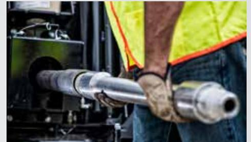
EZ Connect allows operators to change tooling without putting torque on the drill or pipe.
