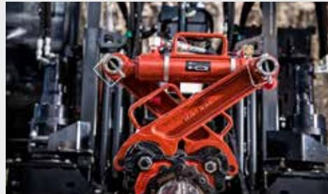
The hydraulic Hydra-Tong is adjustable and works for a range of diameters (3-5/8"-5").
