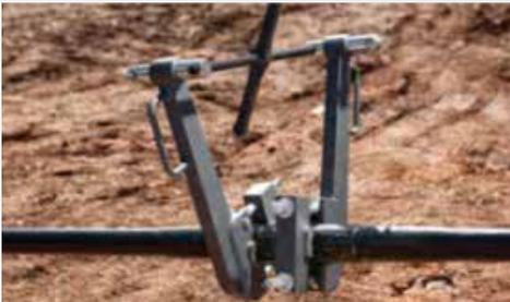
The Quick Wrench is a manually powered wrench that comes in a variety of shapes and sizes.
