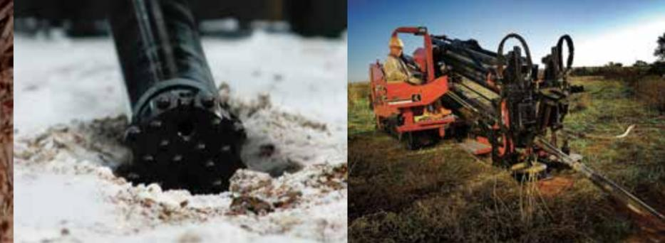
Ditch Witch® All Terrain Directional Drills are so named because they perform with exceptional efficiency in the widest range of ground formations, from mixed hard soil to cobble to solid rock. Equipped with the **All Terrain Air Hammer**, Ditch Witch All Terrain Directional Drills expand this range to include the hardest of rock—20,000 psi and up. More important, the All Terrain Air Hammer expands your productivity.
